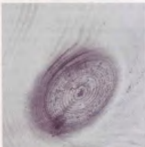
Sound, tight (intergrown), oval red knot.
